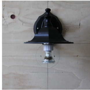
Fig. F.5.4: 50 W TH GU10 in adapter.
