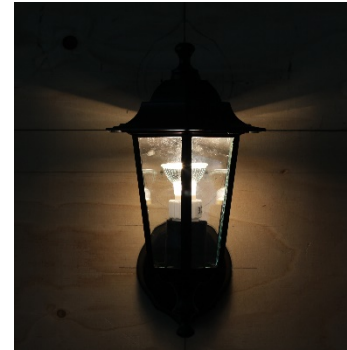
Fig. F.5.9: 50 W TH GU10 in adapter.
